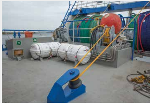
A jumper winch can be used to lift the nets
