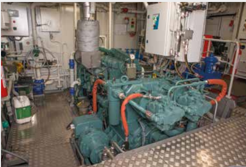
The gearbox is large for a high reduction ratio
