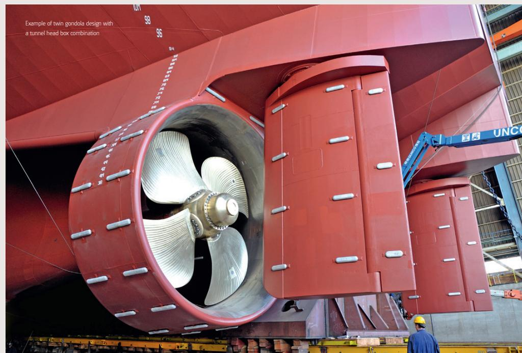
Example of twin gondola design with a tunnel head box combination
